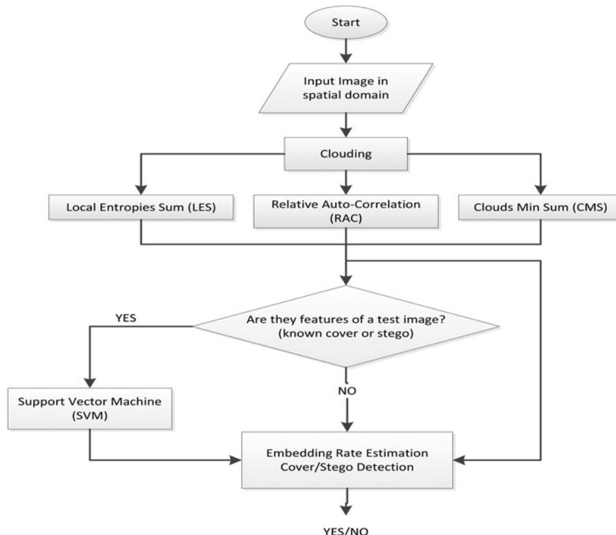
Fig. 1 Flowchart of the proposed steganalysis algorithm
