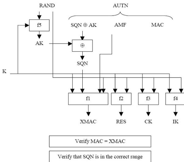
Fig. 3. User Authentication Function in the MS [1]
